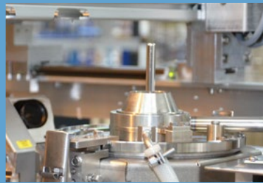
Long solder nozzle for PCBs with high components on soldering side
